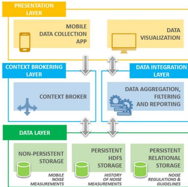
Fig.1 – Platform logical architecture in the large
